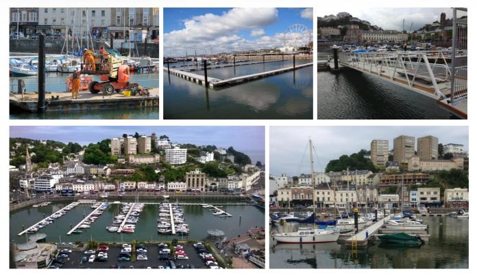
Both galvanised steel and aluminium pontoons, with GRP decking and concrete floats were installed for strength, stability and longevity. The pontoons incorporate a unique side rail profile, enabling the fingers to be quickly adjusted to accommodate larger or smaller beamed vessels. Service pedestals supply water, power and lighting to each berth and access to the pontoons is via a gated linkspan bridge.
